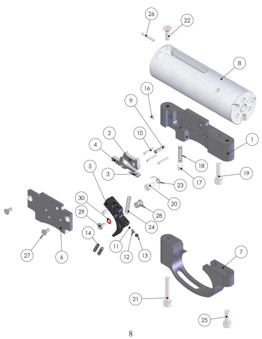
Trigger assembly on the S510 TDR models.
