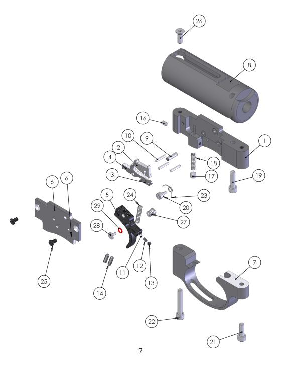
Trigger assembly on the S410 TDR models.
