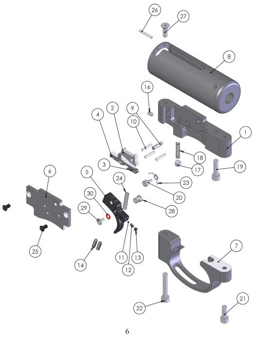
Trigger assembly on the S500 and S510 models including the TC range.
